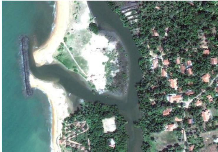
Figure 2 New sea outlet behind the breakwater
